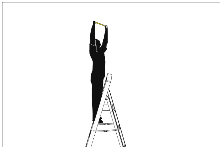
3 Mark mounting spots on ceiling, take care to insure they are in a straight line.
