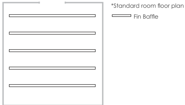
1 Measuring centre to centre, mark the desired placement of Fin baffles on floor.
