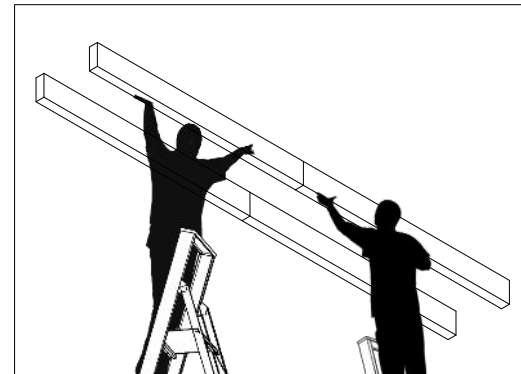
4 Following Step 2-3 as seen on Page 4 , ensure correct Fin-Lock™ alignment and engagement. Repeat for desired array of Baffles
