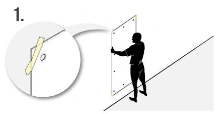
Align stencil to surface of install, attach to wall using a stapler, masking tape or pins. Take that the stencil is flat, it is critical to have precise location of fitments.
