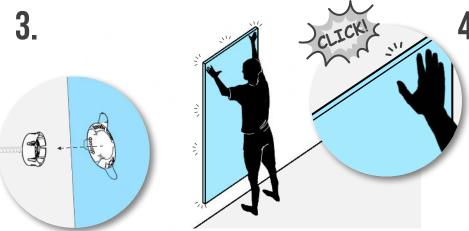
Align acoustic panel, making sure the Male and Female\* Ready-Clips™ are positioned correctly Firmly push at each fitment spot until Clips lock into place.
