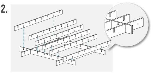
Align 6 x (Part 1) parallel with Part 3. Slide into all slots until flush. When slotting in the fins, push down gently and evenly across length to avoid damage.
