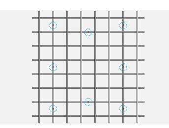
When attaching Matrix to ceiling, push into Direct Fix Clips™ firmly, until they are flush against ceiling surface. They will align with suspension points as marked.
