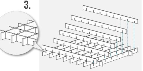
Align 6 x (Part 2) parallel with part 4. Slide into all slots until flush.
