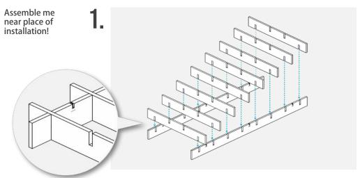
Place 2 x (Part 1) on flat surface. Align 8 x (Part 2) perpendicular to part 1 Slide into all slots until flush.
