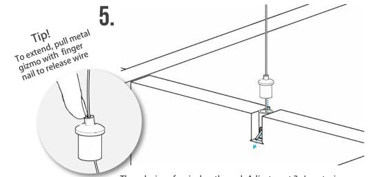
Thread wire a few inches through Adjustment 3. Insert wire through adjustment 4.
