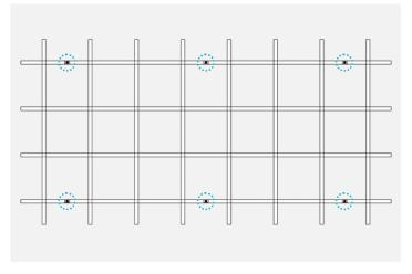
When attaching Matrix to ceiling, push into Direct Fix Clips™ firmly, until they are flush against ceiling surface. They will align with suspension points as marked.
