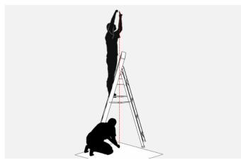
Lay supplied stencil on ground directly below ceiling surface you would like to install your Vista panel.
