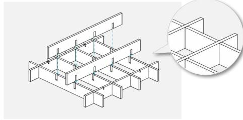
Align 2 x (Part 3) parallel with Part 1. Slide into all slots until flush. When slotting in the fins, push down gently and evenly across length to avoid damage.
